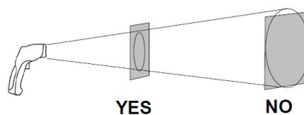
Make sure that the target is larger than the size of the laser sighting.
