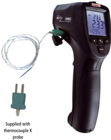
Supplied with thermocouple K probe
